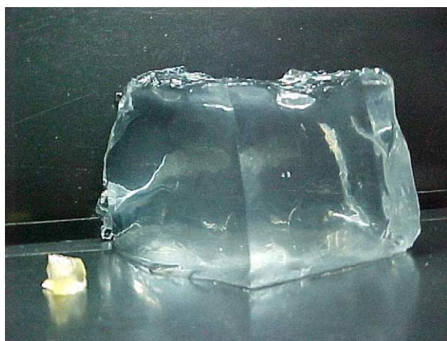
Fig. 12. Photo of (0.4–0.4–4.5) CGMA-co-AAm hydrogel, dried (left side) and swollen (right side).
